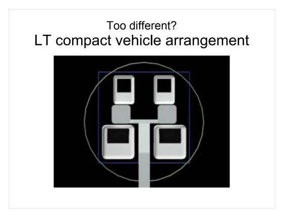
One of the design goals is to run 4 LT lanes inside roadway space, so less than 16 ft (5 m) high and as narrow as possible, to allow building in transitway/busways or even in train tunnels where two lines could mean up to 40,000 pph.
