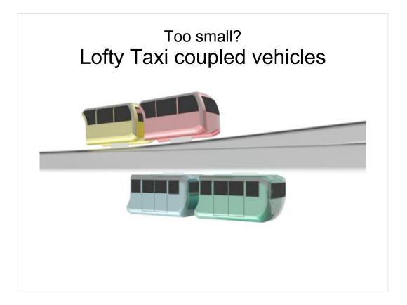
Coupled operation. Coupled operation is where two podcars are virtually linked (they run bumper to bumper) and are only allowed to split up at diverge points where each vehicle leader and follower has its own track and so no possibility of energetic collision. Merging is done at bumper speed typically in stations.
