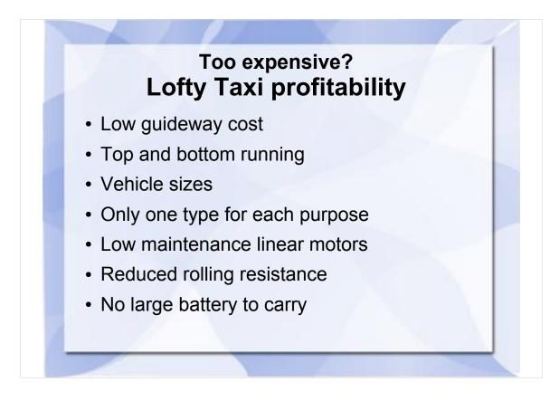
Guideway cost is minimized by using dual-direction guideway. Estimates usually put dual-direction over single-direction at 75% per guideway. So this reduces the cost of the guideway portion, which usually represents 50% of PRT cost, significantly.
