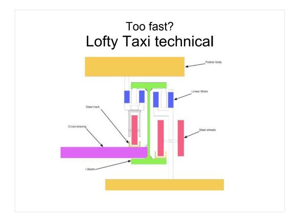
Lofty Taxi uses energy efficient Linear Switched Reluctance Motors instead of small wheels to provide guidance for its vehicles, so high speeds are possible without destroying bearings and wheels, and maintenance is greatly reduced. Switching via dual-sided linear motor is patent pending. Magnetic forces are used to guide a vehicle through a merge or diverge.
